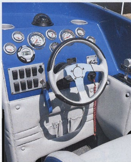
Purpose-cut billet switch panels are flushed into the dash of the Shockwave.
